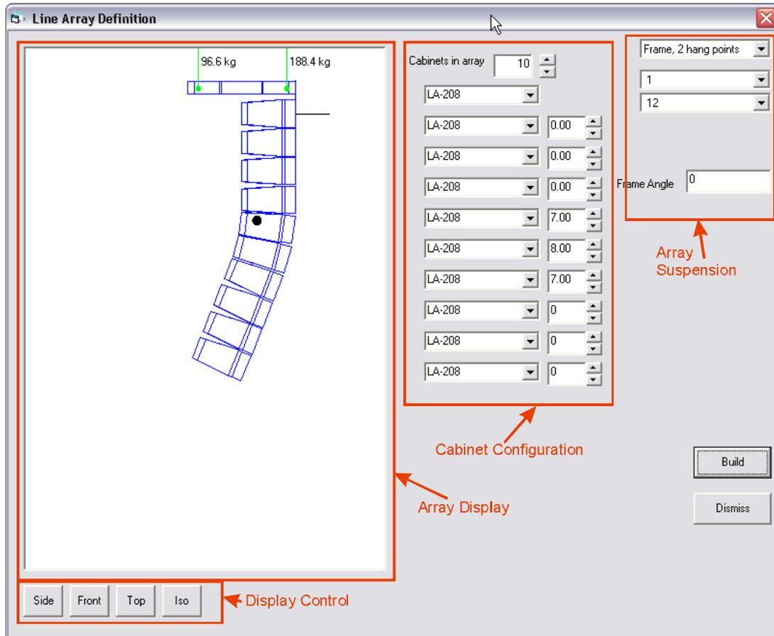
This form is used to define the line array in the room. The controls are in 4 groups, as shown in the figure. The function of the controls is described below. After changing any control, the Build button must be clicked to rebuild the array with the new parameters.
