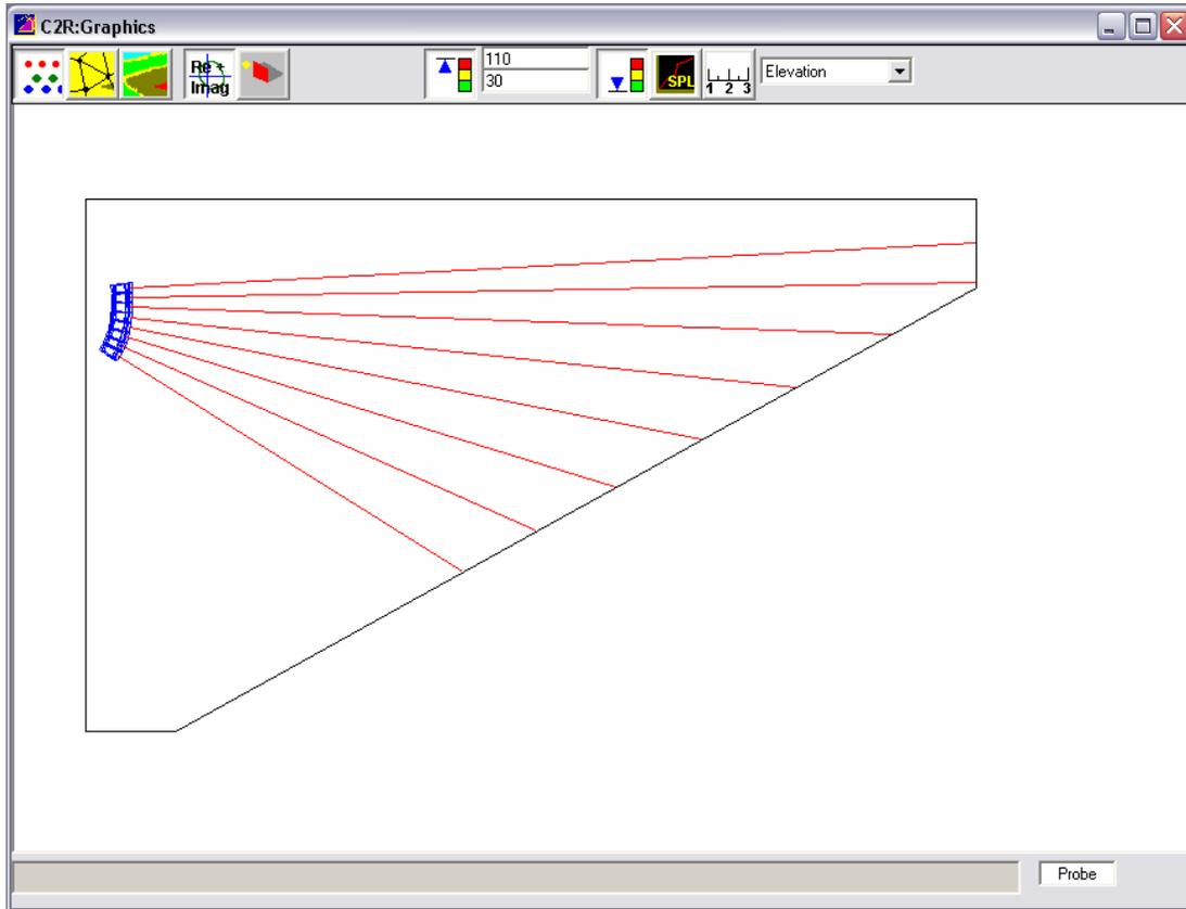
The Graphics Window displays the room geometry and installed loudspeakers. The view is selected from the pull down menu at the top right. This pulldown also selects the surface that calculations will be performed on.
