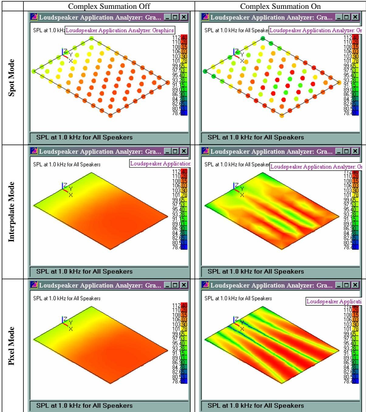
The coverage calculations shown in these displays are performed at a single discrete frequency. This tends to over-emphasise the nulls and peaks shown in pixel mode compared to the perception of a human listening to typical broad band material. The default is to calculate the SPL by averaging over a 1/3 octave band. Selecting 'Calculate at band centre only' on the Preferences form, Listener tab, causes calculations to be performed at band centre frequency only.
