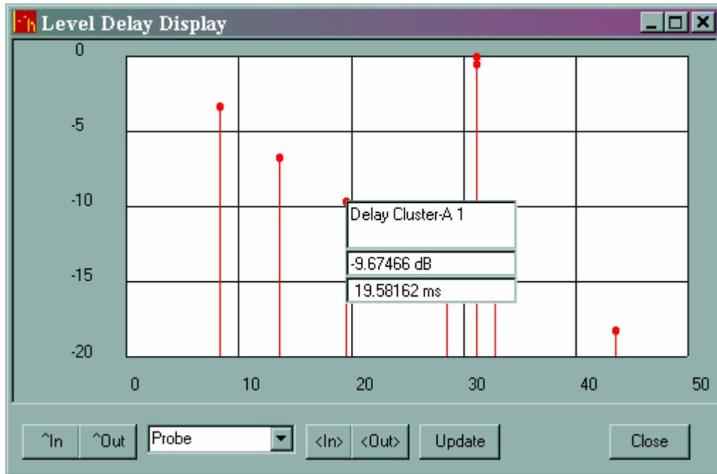
The vertical axis is level in dB, relative to the strongest arrival. The horizontal axis is time in ms.
